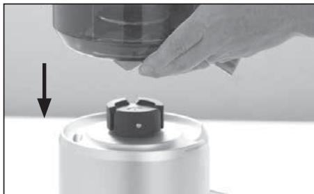
3. Align the arrows at the base of the stainless steel filter basket with the arrows on the motor drive coupling and push down until it clicks into place. Ensure the stainless steel filter basket is fitted securely inside the filter bowl surround and onto the motor base.
