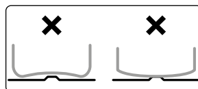
Do not use cookware with concave or convex base. Sensor will not work.
