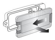
Remove the used bulb by pulling it directly out of its holder.
