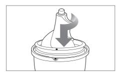
The juicing screw needs to be locked in place in order to close the drum lid.
