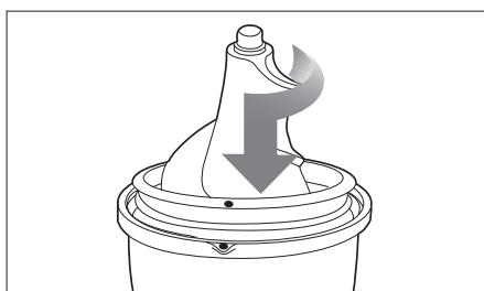
The juicing screw needs to be locked in place in order to close the drum lid.
