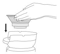
Place the juicer cover over the filter bowl surround, positioning the lower part of the feed chute over the stainless steel filter basket.
