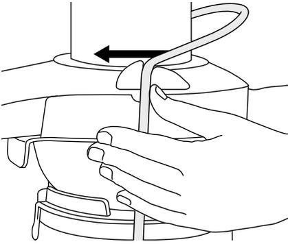
8. Drip stop plug can be fitted over juice outlet nozzle. It then allows the outlet to be plugged to prevent dripping after juicing.
