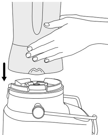
2. Raise the safety locking arm up and locate into the two grooves on either side of the blender.
