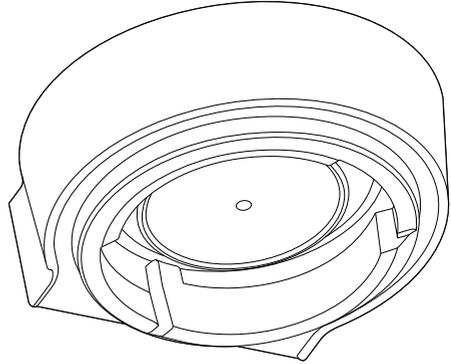
7. Re-insert the shower screen, then the screw. With your fingers, turn the screw clockwise for 2-3 revolutions then insert flat head screwdriver to tighten until the screw is flush with the shower screen. Do not overtighten screw.
