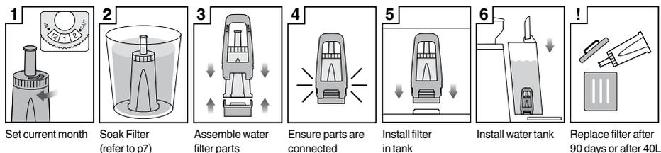
The provided water filter helps prevent scale build-up in and on many of the inner functioning components. Replacing the water filter after three months or 40L will reduce the need to descale the machine.
