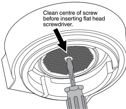
5. Once loosened, carefully remove and retain the screw and the stainless steel shower screen. Make note of the side of the shower screen that is downwards. This will make re-assembly easier. Wash the shower screen in warm soapy water, then dry thoroughly.
