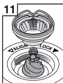
Push upper burr firmly into position
